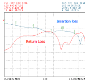
Test Board Insertion Loss
