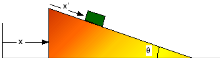
Figure 5: The wedge has mass M and the block has mass m . There is no friction.
